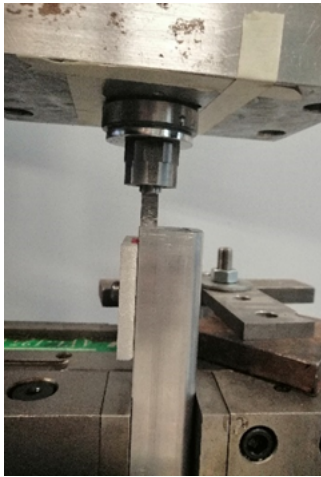
Figure 4. Loaded on screw thread.
